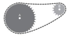
The drive chain is compliant. It can stretch under tension and slacken otherwise. The compliance model consists of a linear spring-damper set in a parallel arrangement. The spring resists tensile strain in the chain. The damper resists tensile motion between chain elements.
