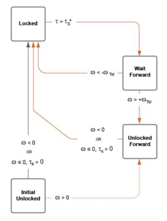
The diagram shows transitions for a two-way clutch.
