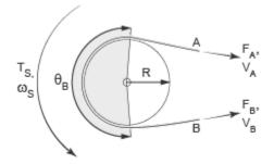
For a flat belt, specify the value of f directly in the block parameters dialog box. For a V-belt, the model calculates the value as
