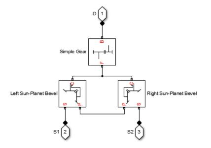
To increase the fidelity of the gear model, you can specify properties such as gear inertia, meshing losses, and viscous losses. By default, gear inertia and viscous losses are assumed negligible. The block enables you to specify the inertias of the gear carrier and internal planet gears only. To model the inertias of the outer gears, connect Simscape Inertia blocks to ports D, S1, and S2.
