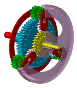
The block models the Ravigneaux gear as a structural component based on Sun-Planet, Planet-Planet, and Ring-Planet Simscape Driveline blocks. The figure shows the block diagram of this structural component.
