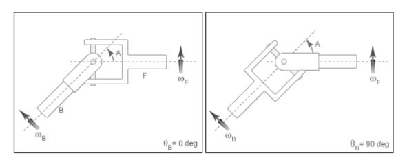
In the figure, the intersection angle is the angle between the two shafts about the pin of the base shaft. The absolute value of this angle must fall in the range  $0 \le A < Ma \times imum$  intersection angle. The base shaft angle is the angle of the base shaft about its length axis. The base shaft angle is also the time-integral of the base shaft angular velocity,  $\omega_B$ .
