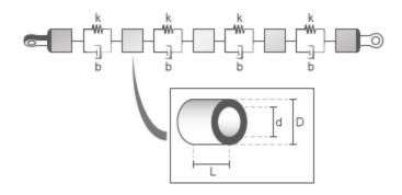
The equivalent physical network contains N segments, each consisting of a spring, damper, and inertia. A segment represents a short section of the driveshaft, the spring represents torsional compliance, and the damper represents material damping. The total shaft inertia is split into N + 1 parts, and distributed evenly along the length of the shaft.
