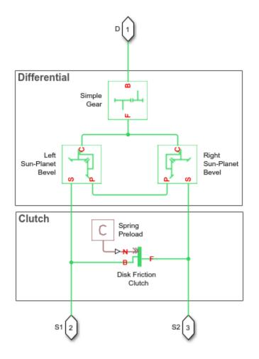
The ports of the Limited-Slip Differential block are associated with the driveshaft (port D) and the two driven shafts (ports S1 and S2), which connect the sun-gears to the wheels.
