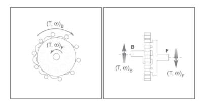
The cycloidal drive can operate in reverse mode, e.g., with power flowing from the follower shaft to the base shaft. In this mode, torque transfer efficiencies are typically negligible. You can adjust the efficiency value in the block dialog box using the **Efficiency from follower shaft to base shaft** parameter.
