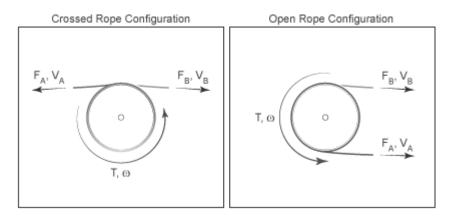
The translational velocities of the two rope ends are functions of the drum radius and angular velocity. Each translational velocity is equal to the tangential velocity of a point at the drum periphery according to the expressions:
