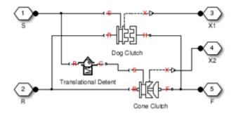
The model implements Dog Clutch, Translational Detent and a modified version of Cone Clutch blocks. Refer to each block reference page for more information on the corresponding block function. You can use a similar approach to model customized versions of the synchronizer. One example is the Transmission (Detailed) subsystem in the model sdl vehicle manual transmission.
