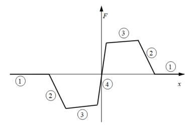
Because the ball is spherical and the notch is symmetric, the horizontal force versus displacement function is symmetric about the origin. (See "Peak Force and Notch Width" on page 1-569.)
